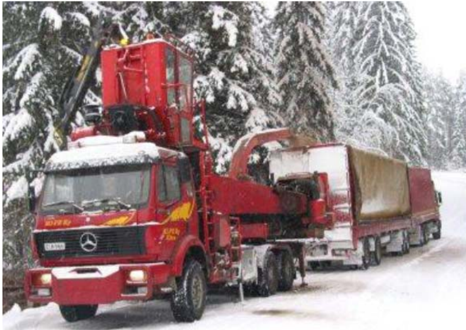
Figure 10: The truck based chipper and chip truck 6
